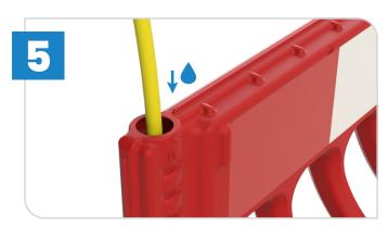
Insert a hose into the open filler hole located at the top of the barrier. Once the barrier, is filled, the barriers weight increases from 5.5kg to 27.5kg.
